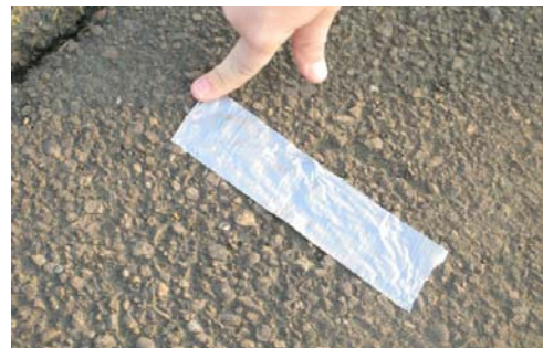
FIGURE 6-68. USE DUCT TAPE TO MEASURE WET FILM THICKNESS OF MARKING.
