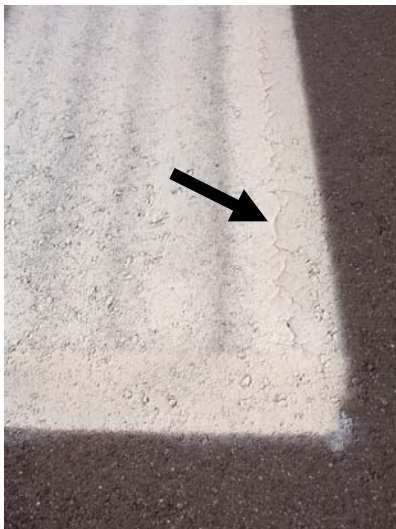
FIGURE 4-11. PAINT CRACKS WHEN APPLIED TOO THICKLY.
