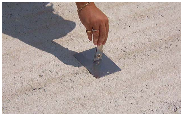
FIGURE 6-67. WET FILM GAUGE ON A METAL COUPON.
