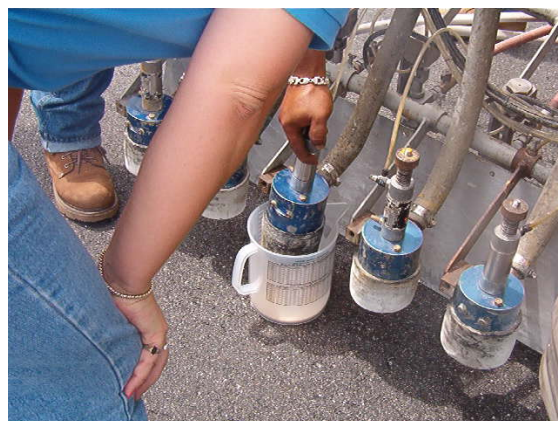
FIGURE 6-60. CALIBRATION OF GLASS BEAD GUNS.
