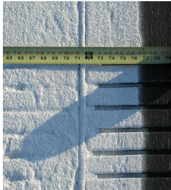
FIGURE 2-3. MARKING DIMENSION IS OUT OF TOLERANCE.
